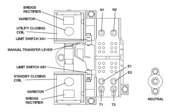
Figure 2.3 — 200 Amp 2-pole Transfer Mechanism
